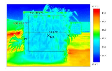
Experiment B: Temperature at Measuring Point 1 (M1) – 31.2°C, 15/08/2019, 12.00 p.m.
