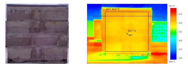
Control Experiment: Temperature at Measuring Point 1 (M1) – 34.7°C, 15/08/2019, 12.00 p.m.
